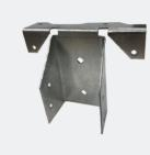
The Ridge to Rafter connector provides alignment control when fixing rafters to the ridge timber and can accommodate any slope up to an angle of 30°.
